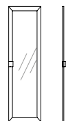
80023 Anta vetro destra per codici 80081/80083/80085/80087/80089/80091 Glass right door for item nr 80081/80083/80085/80087/80089/80091 cm 60 x 2,5 x h 181,5 in 23 5/8 x 1 x h 71 1/2
