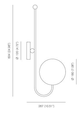
Bulb specifications 240V G9 40W frosted halogen bulb 460 lm / 2800K
