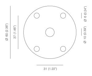
Mounting screws not included. 6mm countersunk screw recommended.
