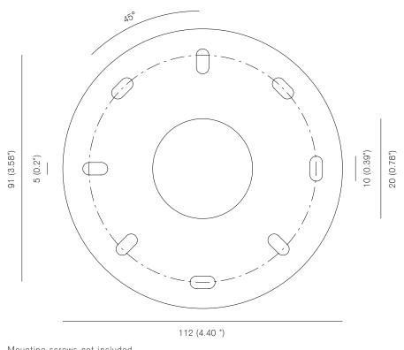
Mounting screws not included. 5mm countersunk screw recommended.
